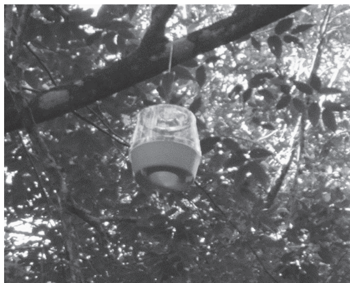
Fig. 1. Multilure trap baited with 300 mL of Streptra Trap® on a tree in the biosphere reserve “El Cielo.”
